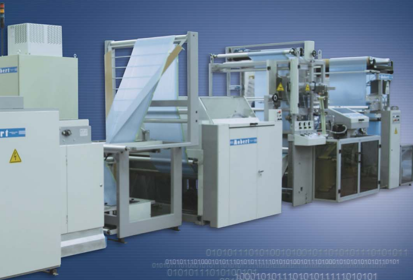
OP 24.1: Guida film. Film guiding system..
